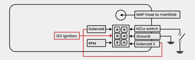
The boost controller will automatically detect a second solenoid and will allow setting Duty up to 200. So basically it works in exactly the same way as before when using duty 0-100% but now duty can be increased up to 200 where the second solenoid starts working. As simple as that. All additional settings for example Boost by RPM or Boost Target will keep working and allow duty up to 200.
