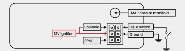
On the back of the unit is a 6 pin connector.
