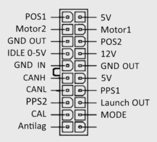
Top 6 pins are connected to the throttle valve. Pre-made wiring loom can be provided for Bosch (VAG) throttle bodies.
